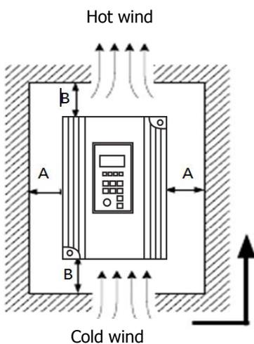
Installation clearance requirements on the MD380 series AC drives of different power classes
